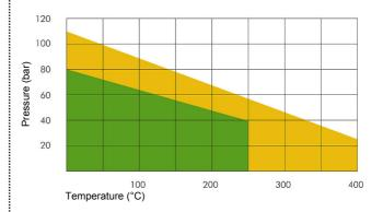
The P x T diagram above indicates the service limits for NA-1002 considering the simultaneous influence of pressure and temperature (chemical suitability assumed). The green area represents the normal service limits, while the orange colored area shows the maximum application limits. For those cases, please consult our technical department.
