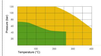
The P x T diagram above indicates the service limits for **NA-1100** considering the simultaneous influence of pressure and temperature (chemical suitability assumed). The green area represents the normal service limits, while the orange colored area shows the maximum application limits. For those cases, please consult our technical department.
